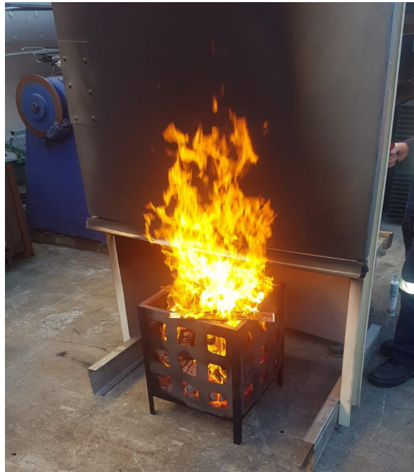
Ceramor coatings passed 60 minute mark for fire retardancy.
