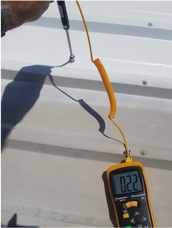
Metal roof application: From 46° C to 22° C.
