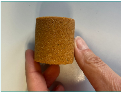
Durocs 1120 mixed with sand. Similar strength to concrete.
